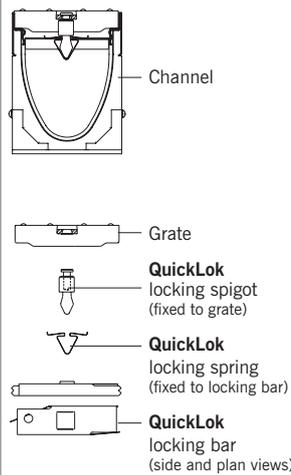
ACO QuickLok is a patented boltless locking system, grates are removed and replaced with the minimum time and effort for ease of maintenance. The unique design provides a positive 'snap down' fit into the locking bar. A spigot is fixed to the grate which 'locks' into the spring in the locking bar.
