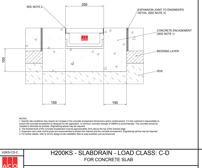
**INSTALLATION DRAWING - ACO DRAIN**
