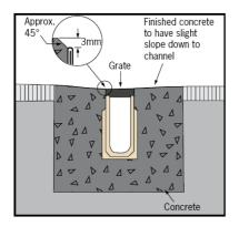
The top of the encasement adjacent to the pavement must be above the grate level (approximately 3mm), this ensures all liquids drain into the channel and that the channel edge is protected against direct traffic loads, see adjacent illustration (left). The same applies for pavements laid up to the channel edge.
